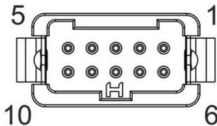
Mating option #1 - connector with latches - G125-FC11005L0-0150L
